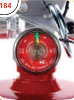
FIRE EXTINGUISHER PRESSURE GAUGE
